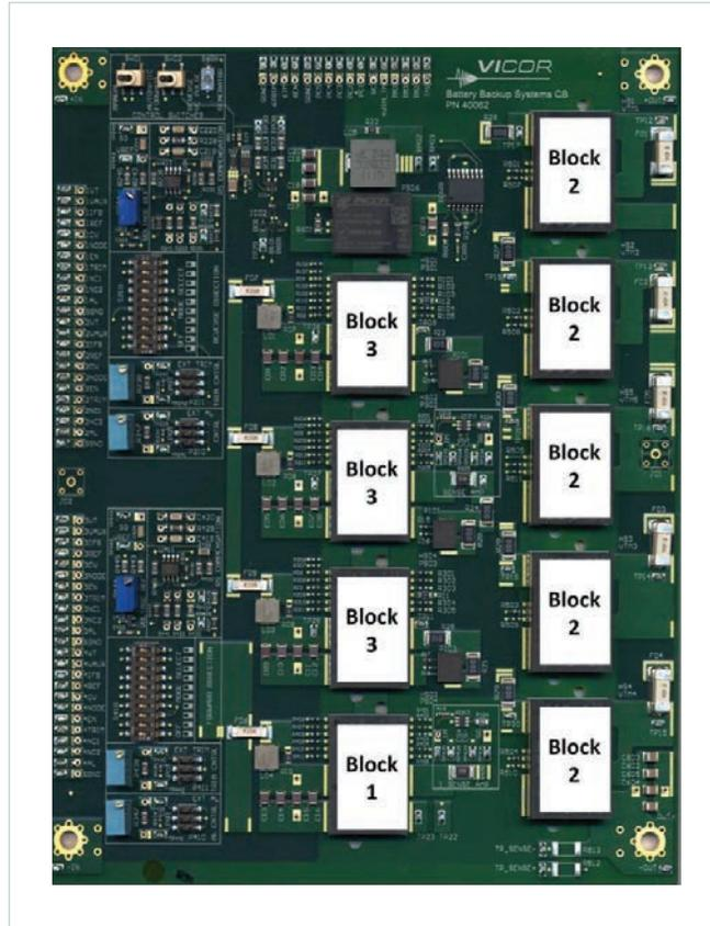
A simple paralleling of modules and putting them together as the topology in Figure 2 would allow this converter to work. Set the regulated  $V_{OUT}$  of the block 3 modules to a relatively low-bus voltage, which is less than normal bus voltage most of the time, but is still sufficient to support the bus load. In this way, no more system control circuitry is necessary. All five block 2 modules can process power immediately once it is in supporting-bus mode.
