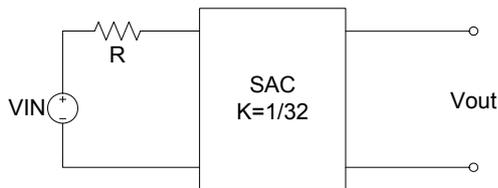
**Figure 3:** Sine Amplitude Converter with series input resistor
