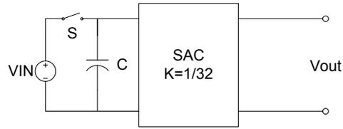
**Figure 4:** Sine Amplitude Converter with input capacitor
