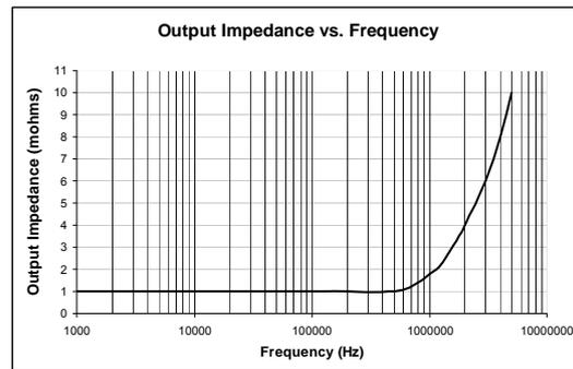
**Figure 5:** Output impedance of  $K=1/32$  SAC vs. Frequency.
