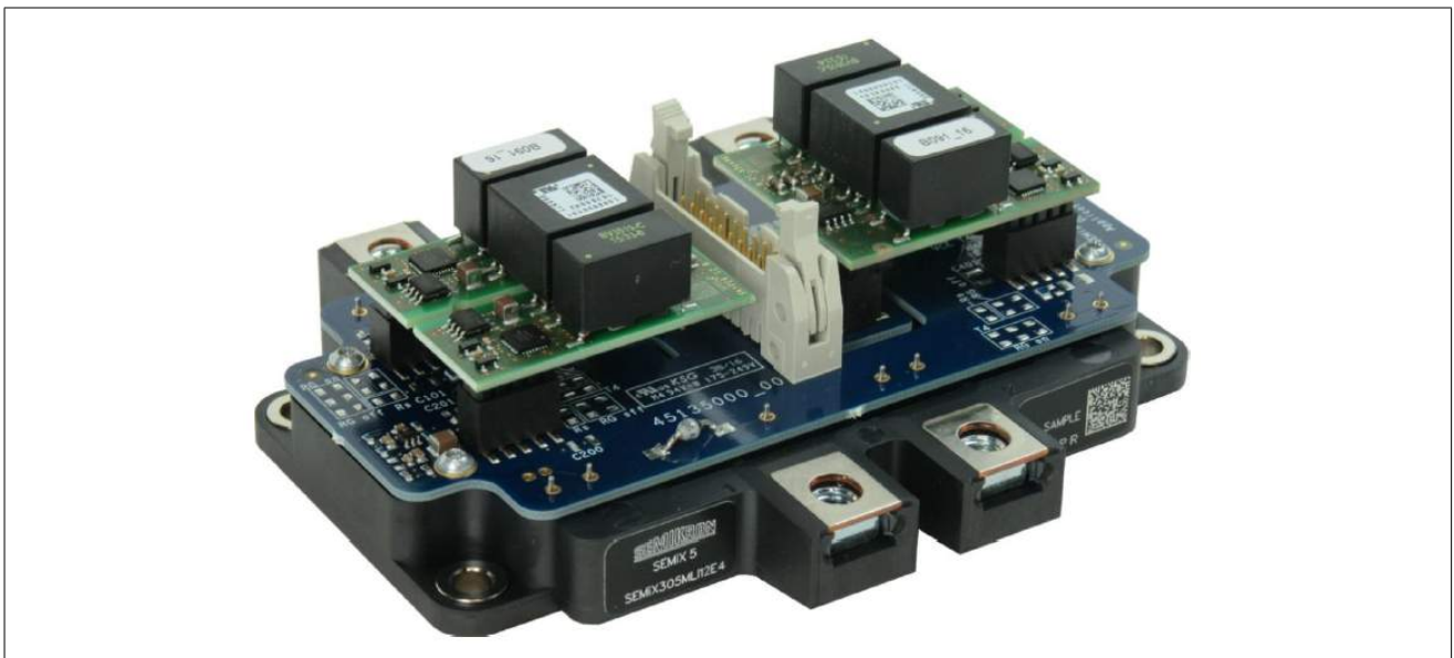
Figure 12: SEMIKRON SEMIX5 TNPC and NPC application sample
