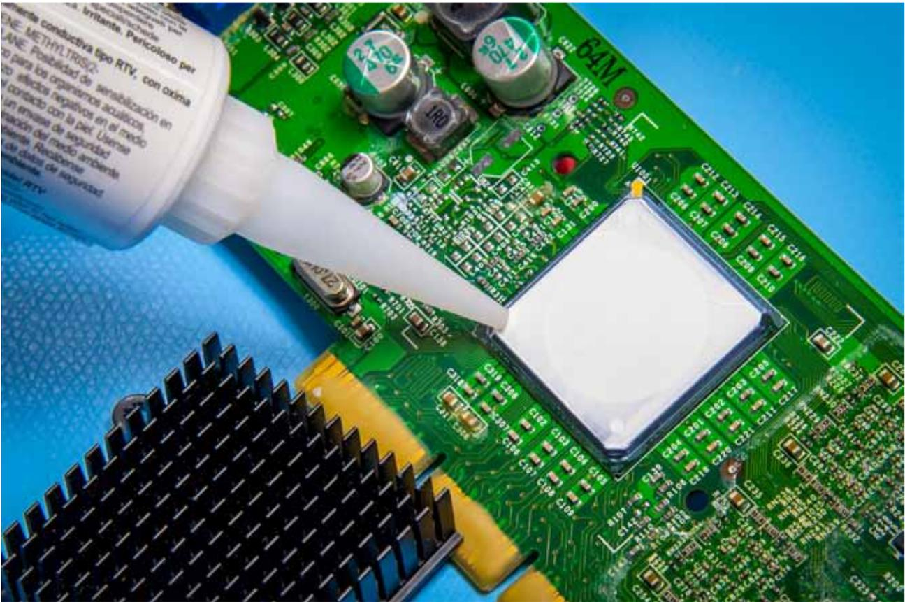
high or low bond strength. High bond strength materials include those based on epoxy chemistry. Other materials may offer a range of properties to meet the individual application requirements. For example, Electrolube's new silicone RTV, TCORP, offers the best combination of viscosity, operating temperature range, thermal conductivity and bond strength for electronic applications.
